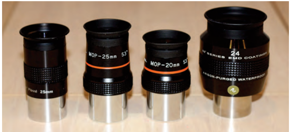
Image 8 – The 25mm and 20mm were compared to a 25mm Plössl and a 24mm 68° Explore Scientific eyepieces.
