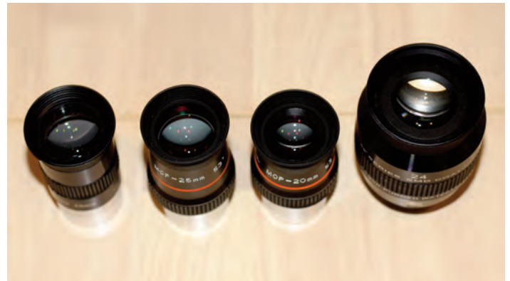
Image 9 – A top view of the 25mm MOP, the 20mm MOP, the 25mm Plössl, and the 24mm 68° Explore Scientific eyepieces. All four have approximately the same diameter opening.
