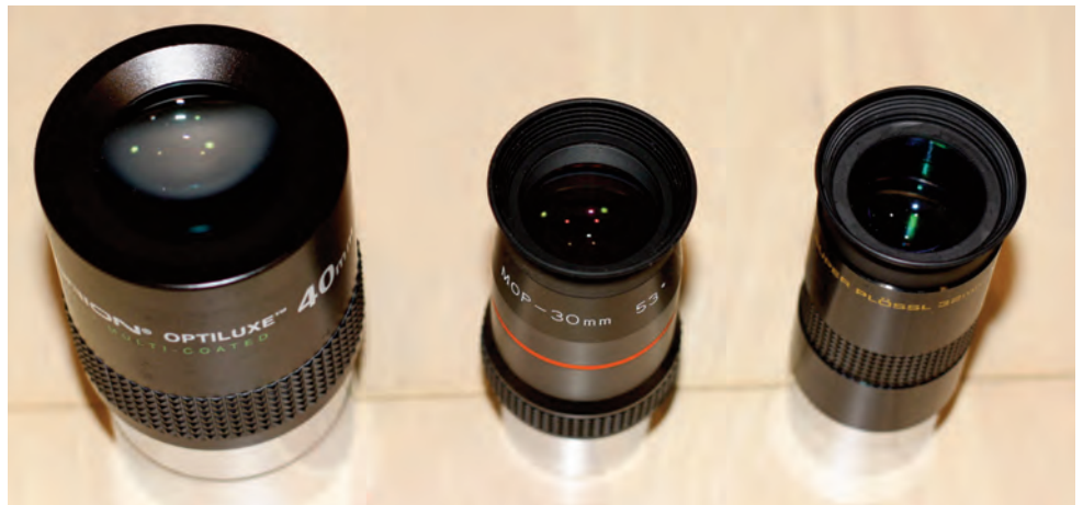
Image 7 – A top view of the 30mm Masuyama Ortho Plössl, the Orion Optilux, and the Meade 32mm Super Plössl eyepieces showing the glass in each.
